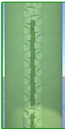
Step: 3 Insert 2 nd key same as the 1 st and continue procedure until all keys are fitted.
